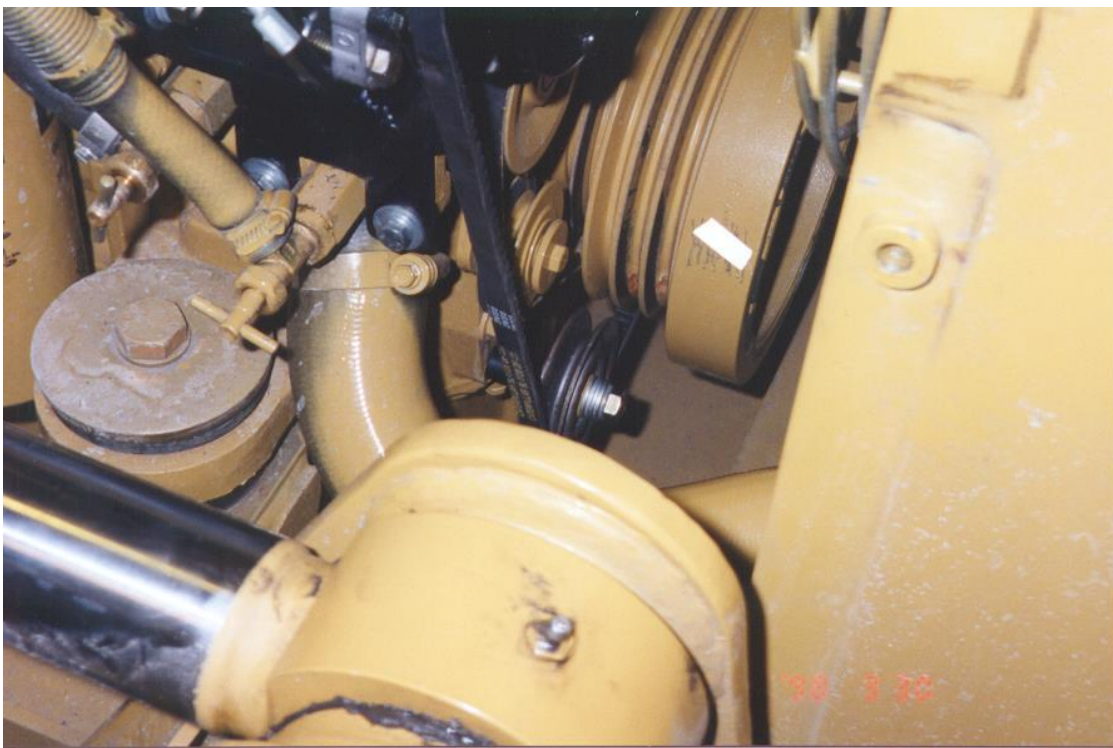
Compressor mount and drive with idler pulley.
