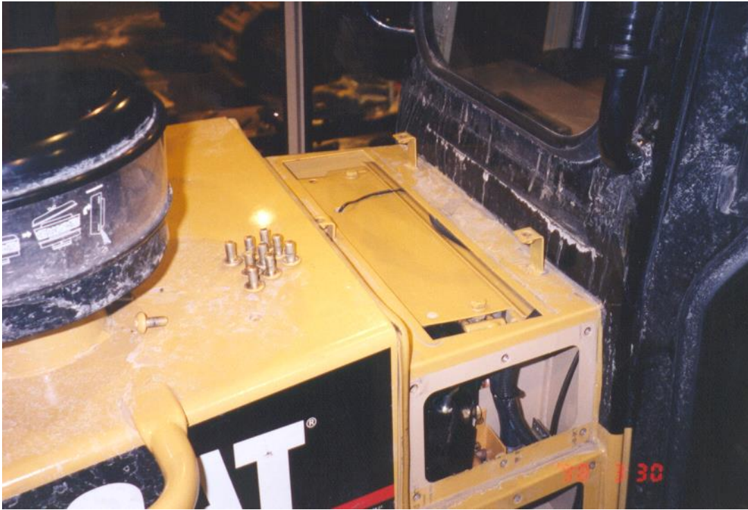
Evaporator cover in place with thermostat.
